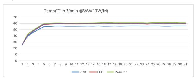
The above curves indicate the temp. changing in Resistor, LED, PCB within 30 minutes after powering on, under the ambient temperature of 25  $^{\circ}$ C.
