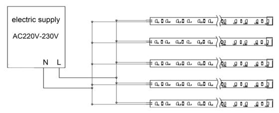
\* Make sure of the total watts of LED Strip lights is less than 80% of the power supply's max output.
