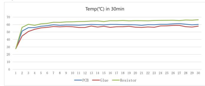
The above curves indicate the temp. changing in resistors, glue & PCB within 30 minutes after powering on, under the ambient temperature of 25  $^{\circ}$ C.
