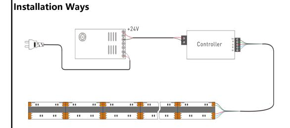
\* Make sure of the total watts of COB Strip lights is less than 80% of the power supply's max output.
